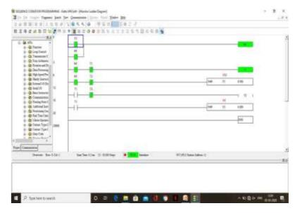
In meantime the Timer (T2) i.e. {TMR T2 K200} will act and when the Robot work will completed the timer get over and it automatically stops and again the process continues going.
