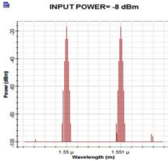
Fig 4.3 The optical spectrums at the output when the two wavelengths are transmitted at -8dBm.
