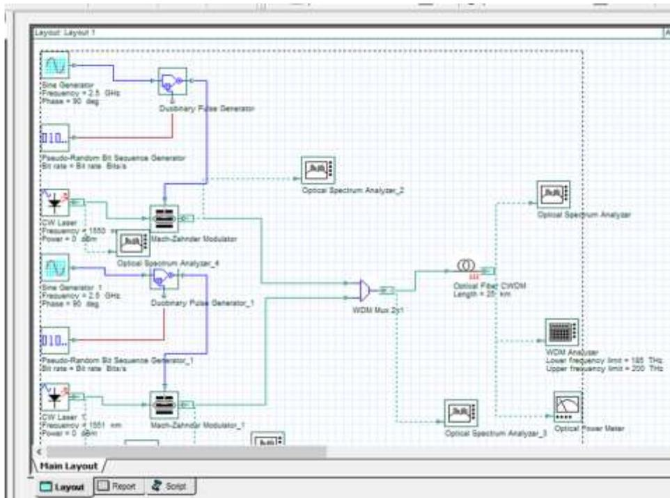
Fig. 3.2 FWM simulation set up in Optisystem
