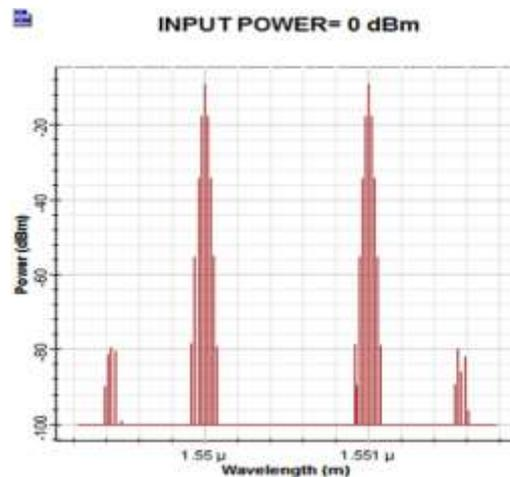
Fig 4.1 The optical spectrums at the output when the two wavelengths are transmitted at 0dBm.
