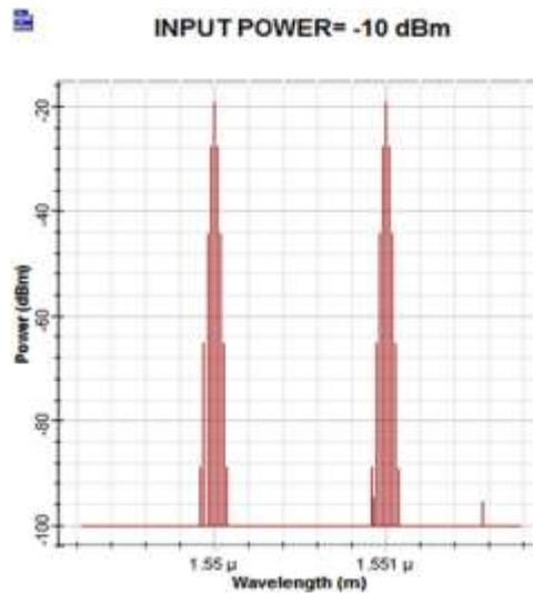
Fig 4.4 The optical spectrums at the output when the two wavelengths are transmitted at -10dBm
