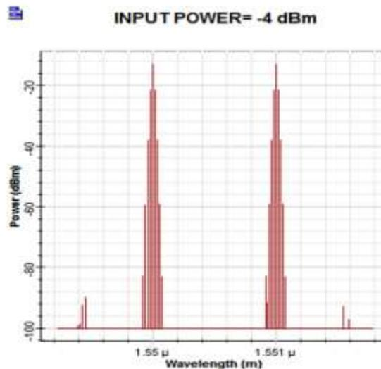
Fig 4.2 The optical spectrums at the output when the two wavelengths are transmitted at -4dBm.
