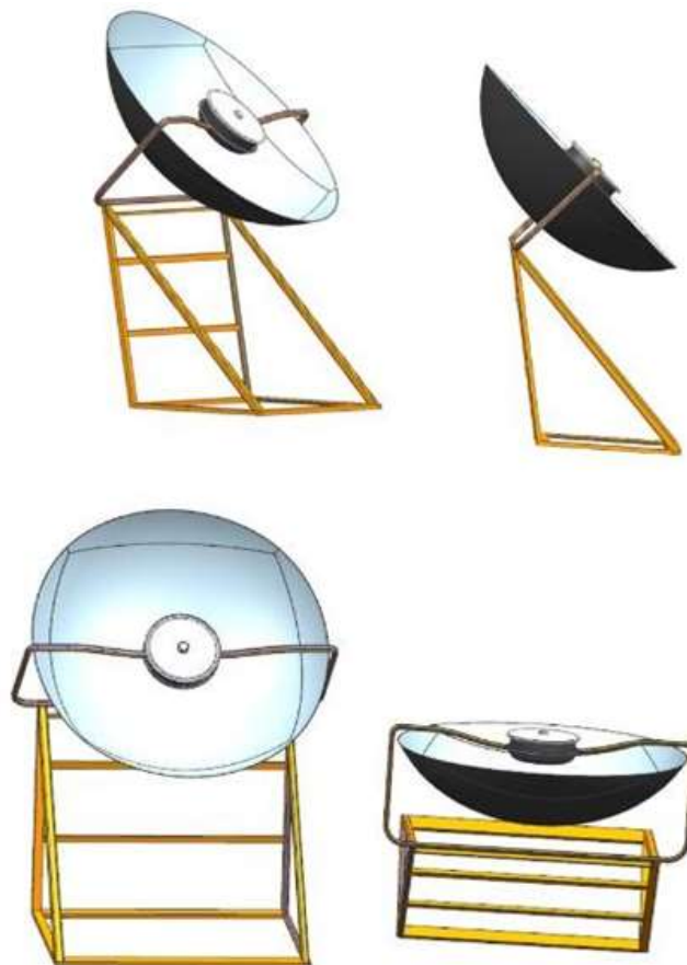
Figure 2. 3D advance modeling and simulation of cylindrical panel solar cooker
