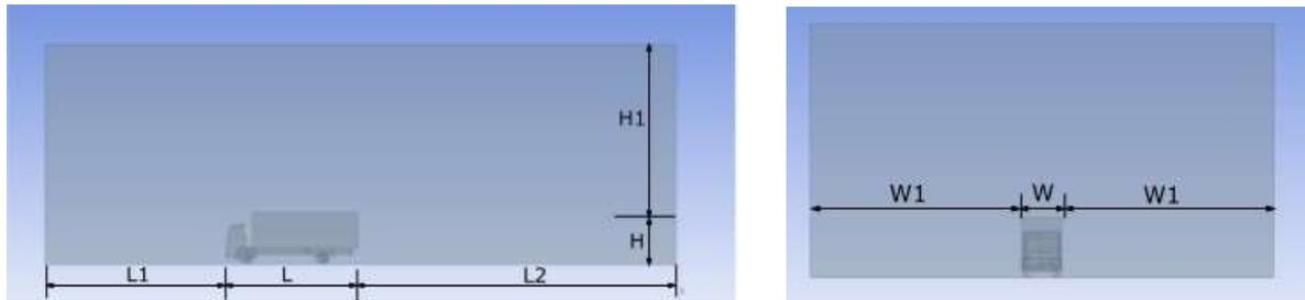
Figure 2: Size of wind tunnel enclosure.
