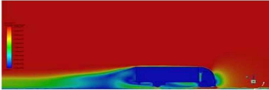
Figure 11: curved cap roof deflector  $R = 1.5$  [m] with curved boat tail  $R = 0.9$ [m]
