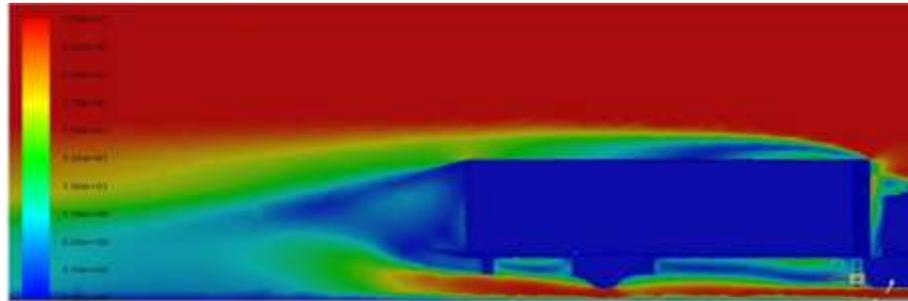
Figure 8: Side view of velocity contours for flat tail boat at angle 20 [deg].
