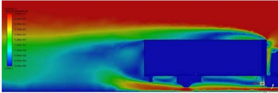
Figure 7: Side view of velocity contours for baseline truck.
