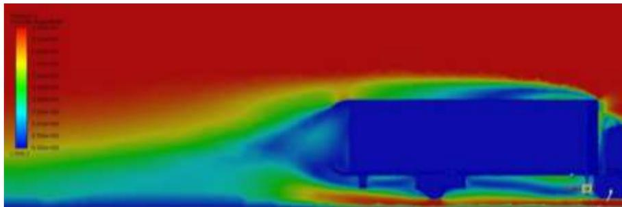
Figure 9: Side view of velocity contours for curved tail boat with 100 [mm] radius.
