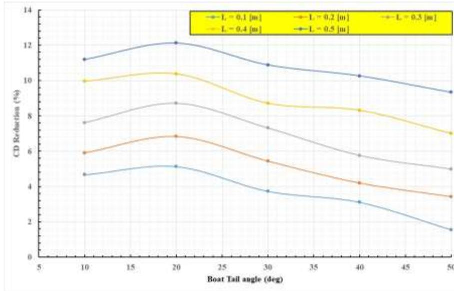
**Figure 5: The drag reduction for the flat boat tail at different angles.**
