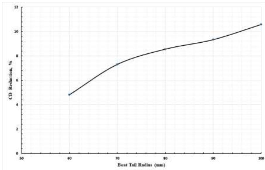
**Figure 6: The drag reduction for the curved boat tail at different radii.**
