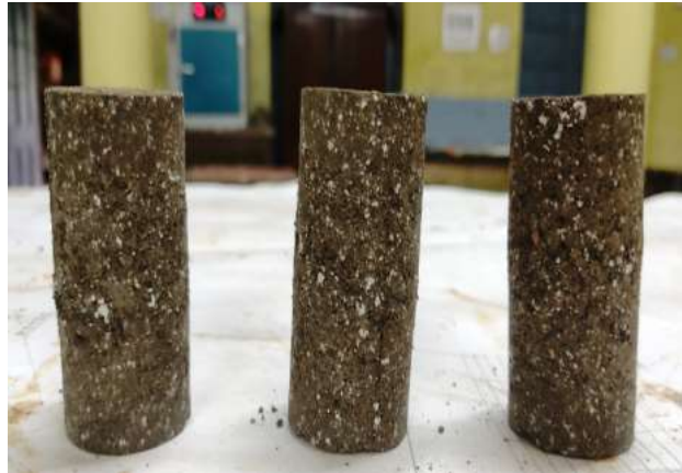
Figure 2. Sample of Unconfined Compressive Strength Test
