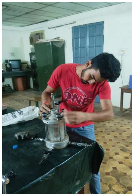
Figure 3. Sample preparations of Unconfined Compressive Strength Test
