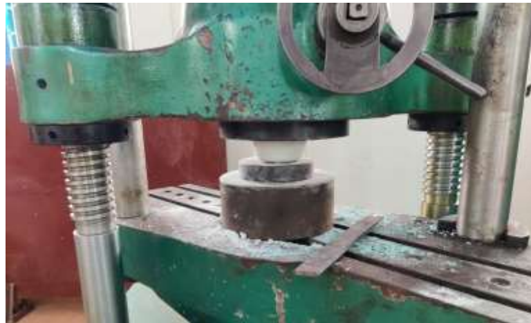
Fig 3. This figure shows compressive strength testing of the sample collected
