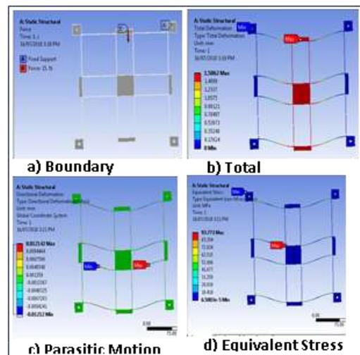
Fig. 4 - Y Directional Deformation of XY Flexural Mechanism 1
