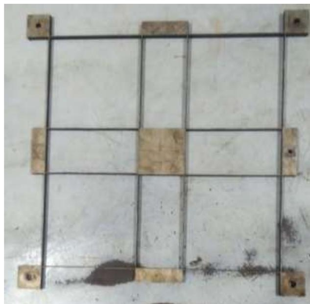
Fig. 5 - Manufactured XY Flexural Mechanism 1
