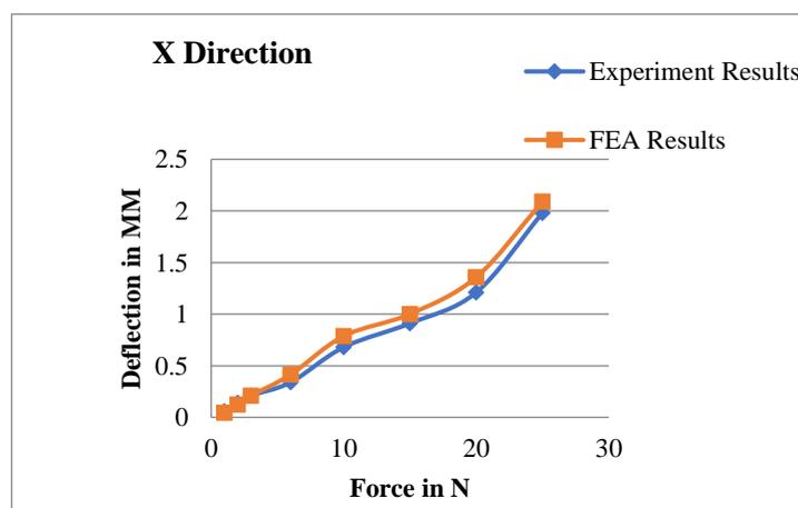
**Fig. 8 - Comparison of experimental and FEA for results for X-direction.**
