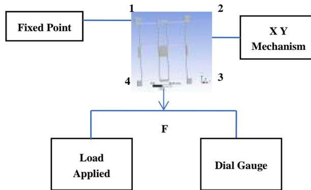
**Fig. 6 - Experimental Setup for Measurement of X & Y Direction motion and parasitic motion**
