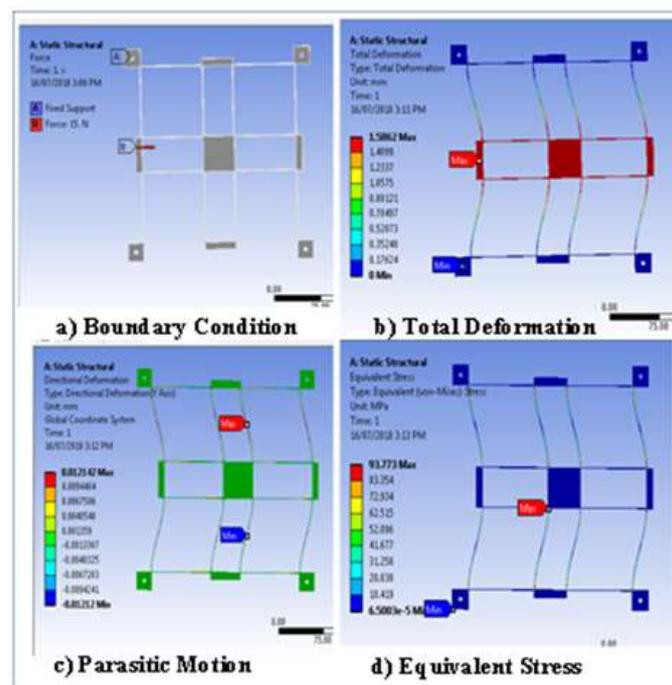
**Fig. 3 - Static Analysis of XY Flexural Mechanism 1**
