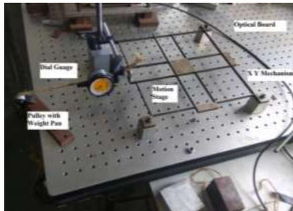
**Fig. 7 - Experimental Setup for Measurement of X & Y Direction motion and parasitic motion**
