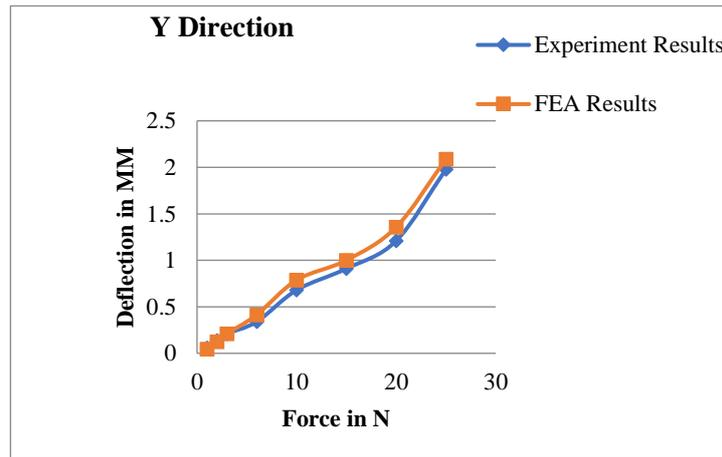
Fig. 9 - Comparison of Experimental and FEA results Y-direction
