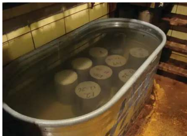
Fig 2: Curing concrete specimen
