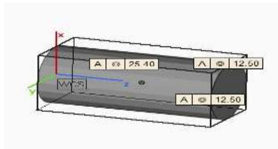
**Figure 3.7: Compression specimen of horizontal orientation**
