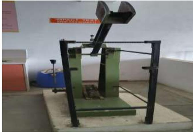
**Figure 3.9: Charpy impact test machine**
