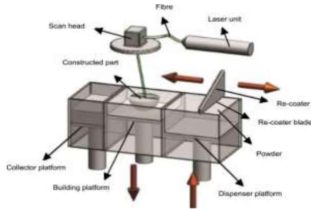
**Figure 1.1: Schematic Diagram of DMLS**
