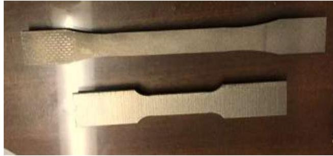
**Figure 3.6: Tensile Inconel specimens**
