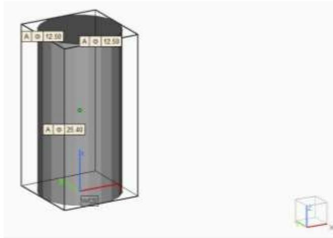
**Figure 3.8: Compression specimen of vertical orientation**
