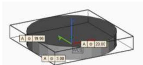
Figure 3.16: Corrosion specimen of horizontal orientation
