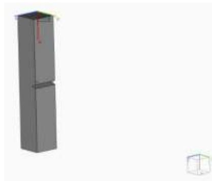
**Figure 3.11: Impact specimen of vertical orientation**
