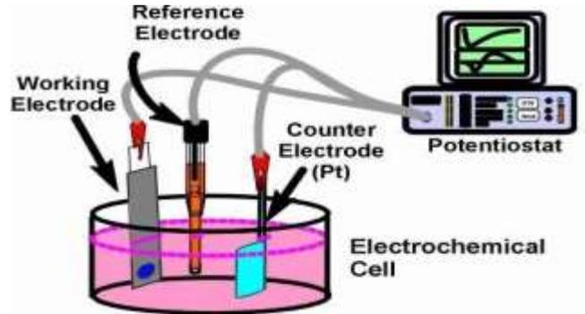
Figure 3.15: Schematic diagram of corrosion test
