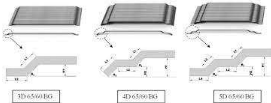
Fig. 3 (a) 3D steel fibre, (b) 4D steel fibre, (c) 5D steel fibre
