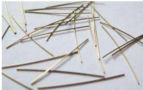
Fig. 1 Straight steel fibres
