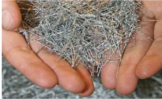
Fig. 2 Deformed steel fibres
