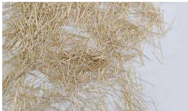
Fig. 4 Micro steel fibres.
