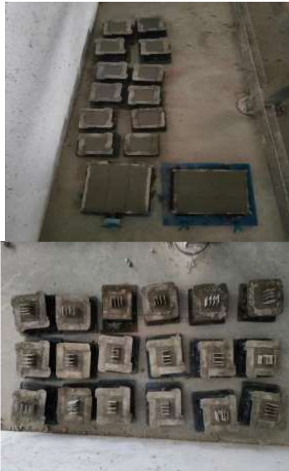
Figure 28 Incorporation of steel plate in specimens-
