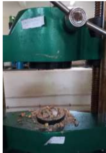
Figure 1.9: Compressive strength test of pavement specimen
