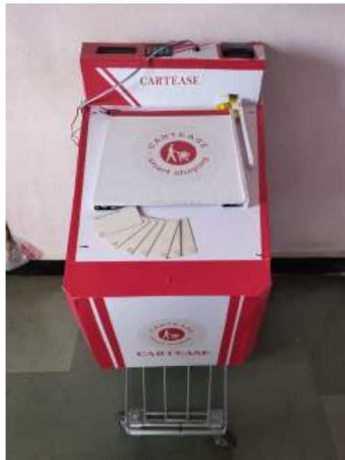
Fig.9. Smart Shopping Trolley using Automated Billing System
