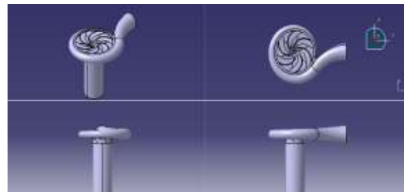
Figure 4: Multi-view of type-2 Design of centrifugal pump
