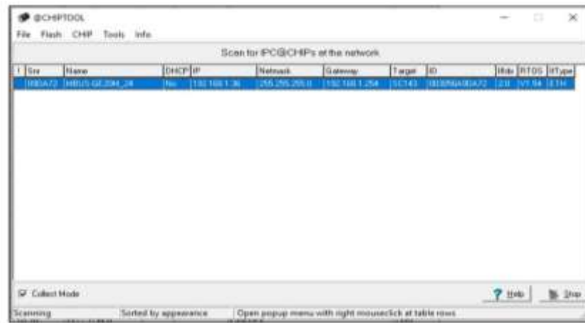
Fig. 4: Overview of the CHIPtool Displaying All Detected MBUS-GEM Devices in the Local Network
