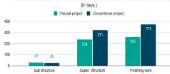
Time comparison between precast and conventional systems
