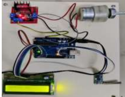
Fig.3. Receiver circuit when the transmitter sends green signal
