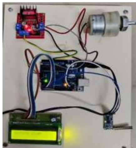
Fig.5.Receiver circuit when the transmitter sends red signal
