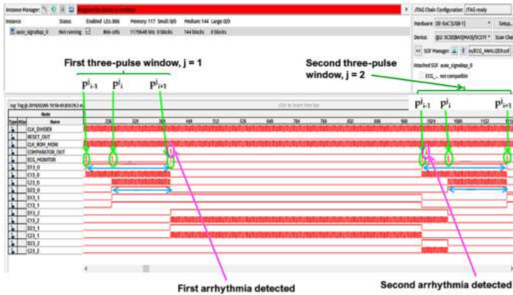
Figure 7. Arrhythmias detection by instrumental analysis performed using the Signal Tap II Logic Analyzer.
