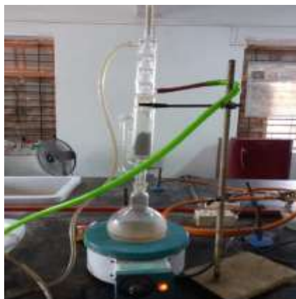
Fig 14. Soxhlet extraction of curcumin
