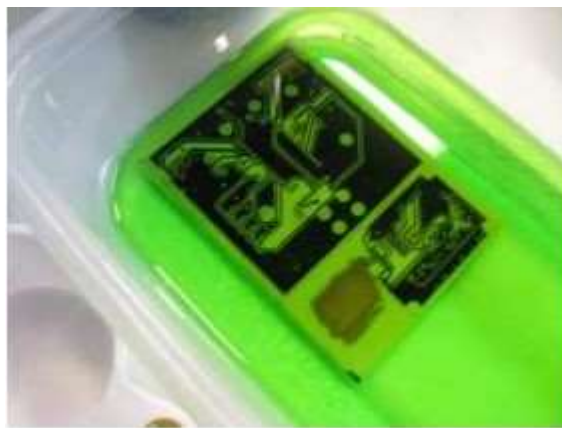
Fig 2: Dissolved copper in the acid bath turned the solution green [2]
