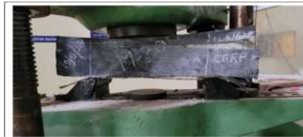
Fig 7-U Shaped Wrapped Cfrp Rc Beam
