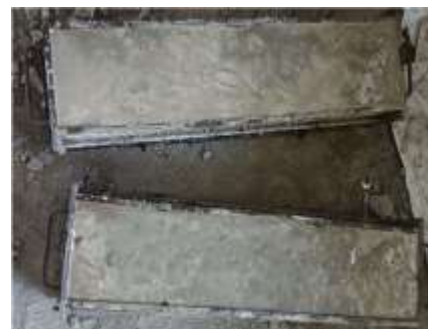
Fig 3-Casted specimen for CFRP Beam
