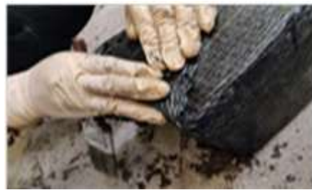
Fig 5-CFRP Strengthened RC Beam (SB-2)
