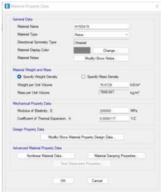
Figure 2.1 Defining Properties of Rebar HYSD 415
