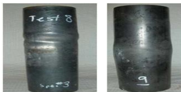
FIGURE.1.2 OUTWARD BUCKLING OF CFST STUB COLUMNS
