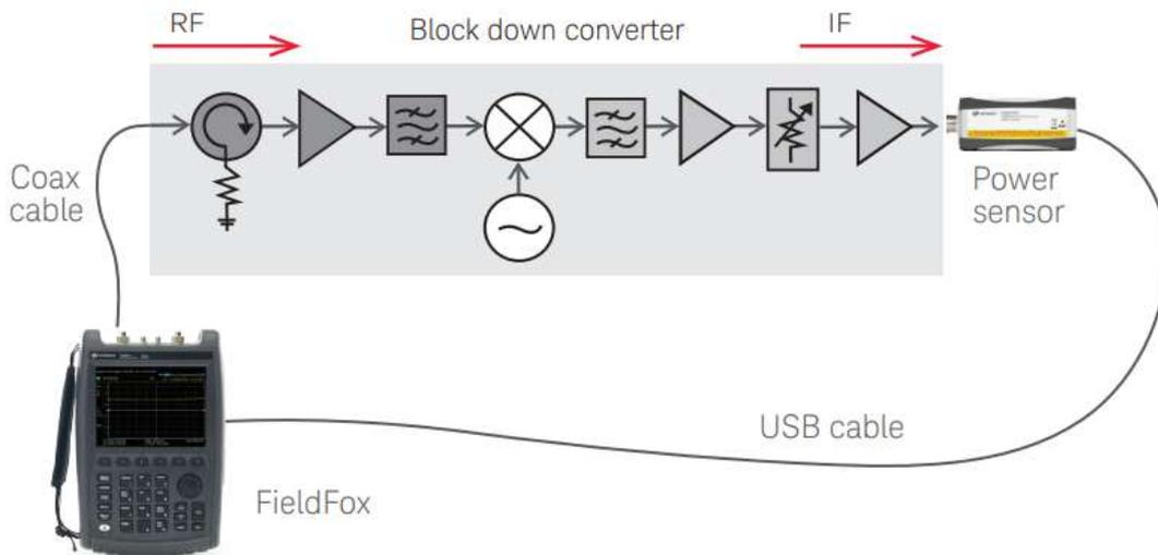
Figure 9 : Frequency block downconverter and associated test configuration [2]
