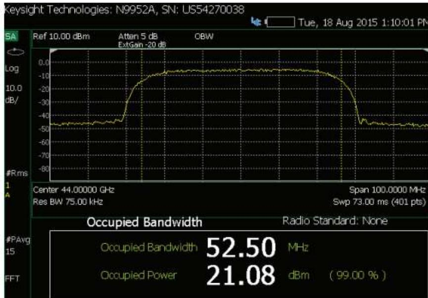
Figure 6 : Measurement of the spectrum and occupied bandwidth from a 44-GHz digitally-modulated input signal [2]
