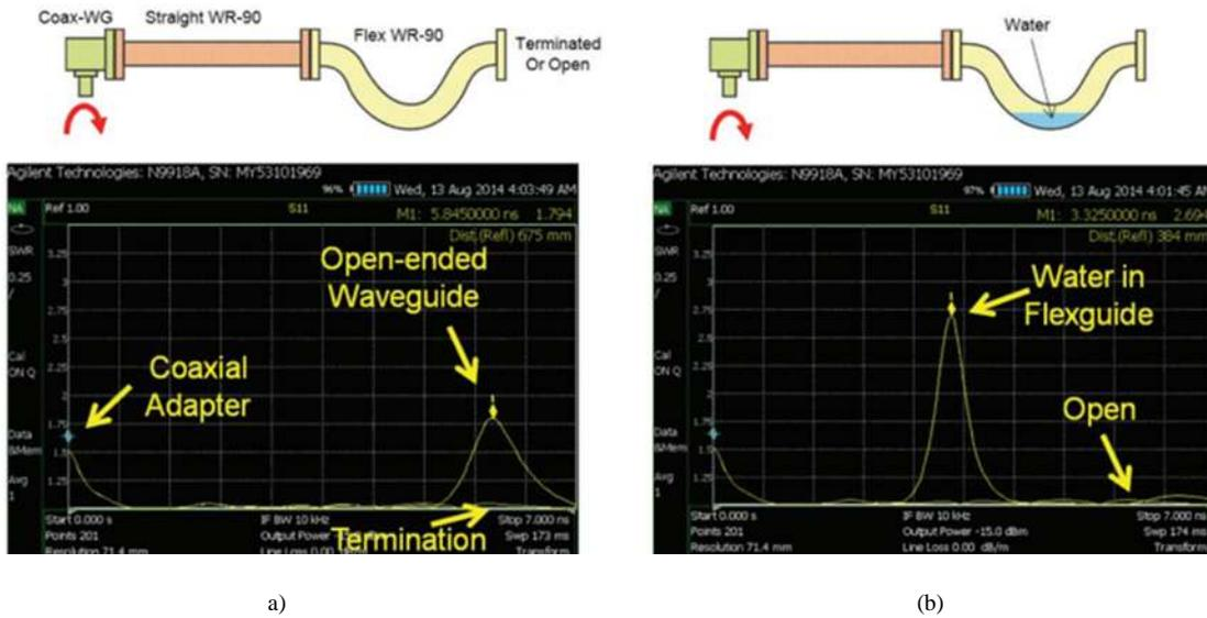
Figure 5 : Time domain measurements of a system of waveguide components [2]
