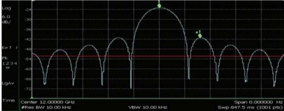
Figure 4: Measured antenna pattern using FieldFox configured in zero span mode with max hold [2]
