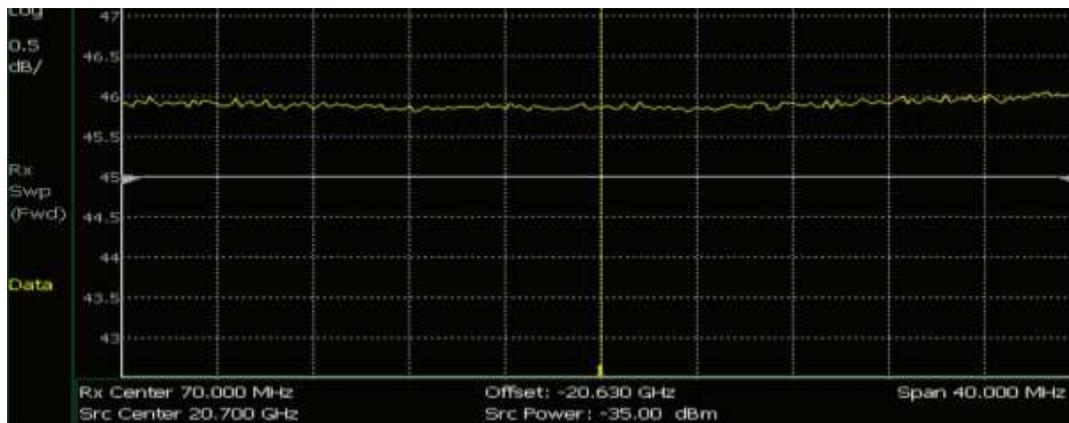
Figure 10 : Measurement of the conversion gain for a Ka-band to 70 MHz earth station downconverter[2]
