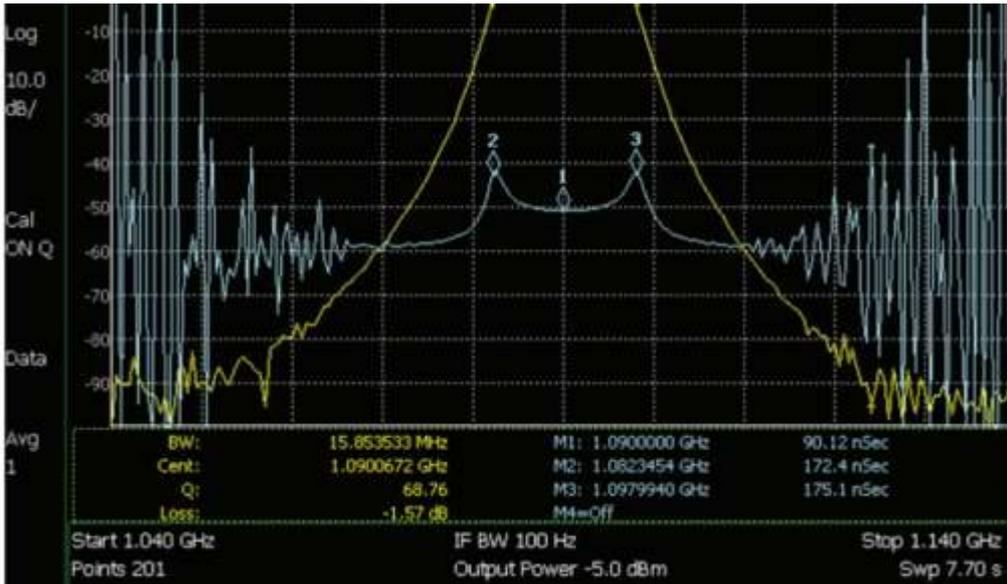
Figure 8: Measured transmission response of band pass filter [2]
