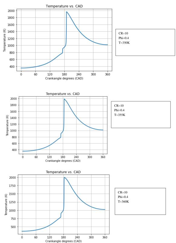
Heat Release Versus Crank degrees at defined compression ratio & Equivalence ratio & Temperature
