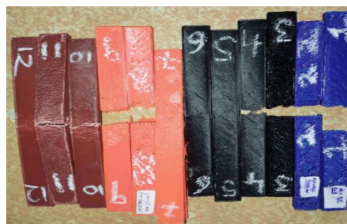
Fig: Flexural specimens after fracture
