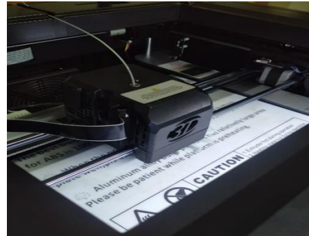
Fig: 3D printed wire, nozzle and heated bed
