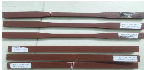
Fig: Tensile and Bending specimens of PETG composites
