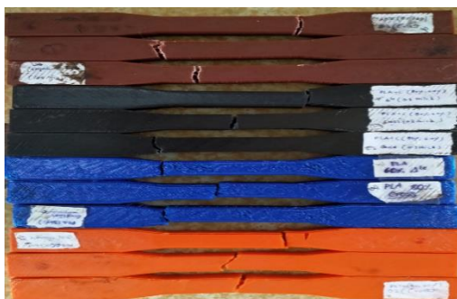
Fig: Tensile specimens after fracture
