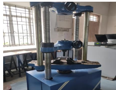
Fig: Universal Testing Machine(Flexural SET-UP)
