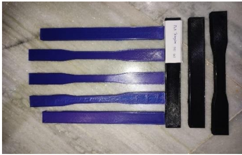
Fig: Tensile and Bending specimens of PLA composites
