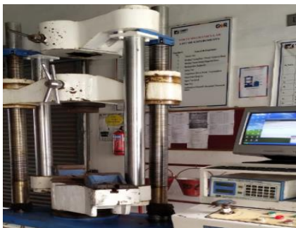
Fig: Universal Testing Machine(Tensile SET-UP)
