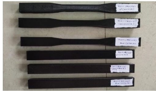
Fig: Tensile and bar specimens of PLA + C composites
