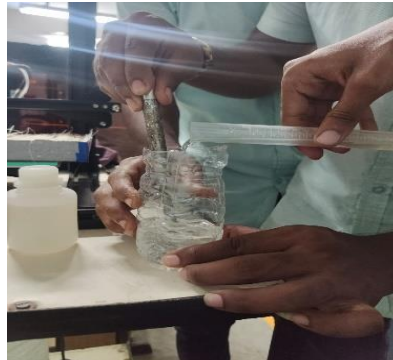
pouring the 100ml resin in a bottle and thoroughly stirring with 10ml of Hardener.
