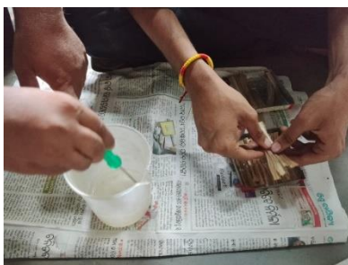
Taking 100ml of resin in a Breaker and 10ml of hardner.
