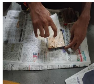
pouring epoxy resin mixture on the 1 st layer
