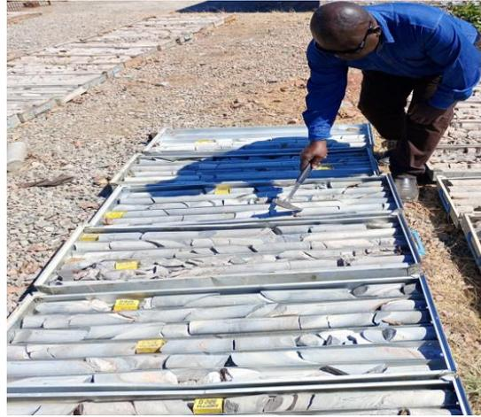
Figure 2: Logged borehole for RQD determinations.
