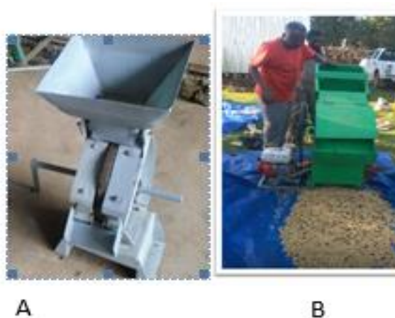
Fig. 1 – (A). Manual operated single disc coffee pulper, (B). Modified engine driven Double disc coffee pulper.
