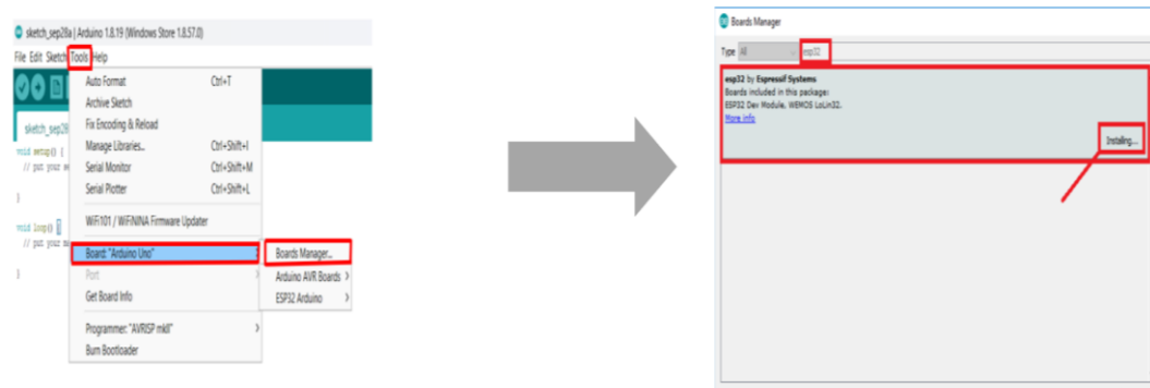
Fig.4.2: Installation of ESP32 Board Manager
