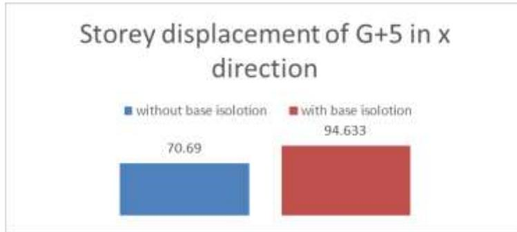
Fig 31: Story displacements of 5 stores in the x-direction
