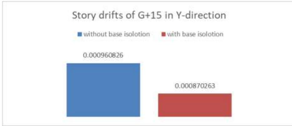
Fig 19: Story drifts of 15 stores in the y-direction
