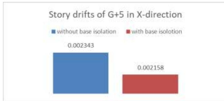
Fig 38: Story drifts of 5 stores in the x-direction
