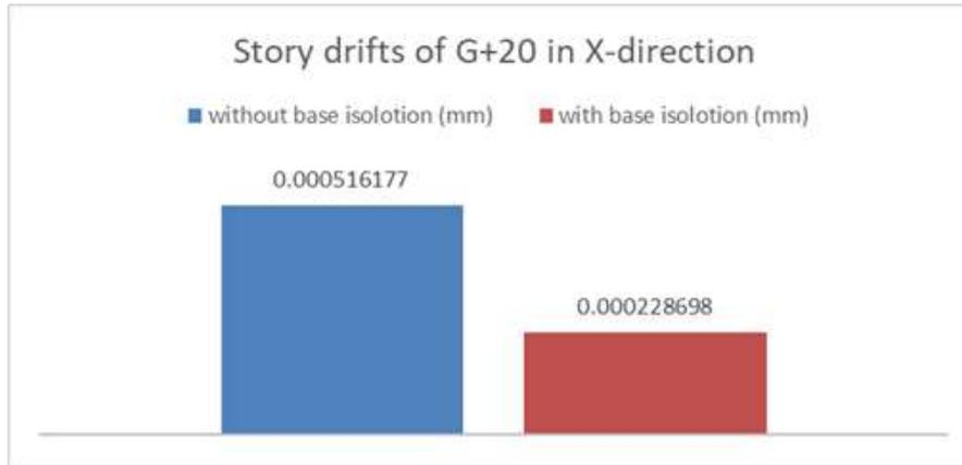
Fig 8: Story drifts of 20 stories in an x-direction
