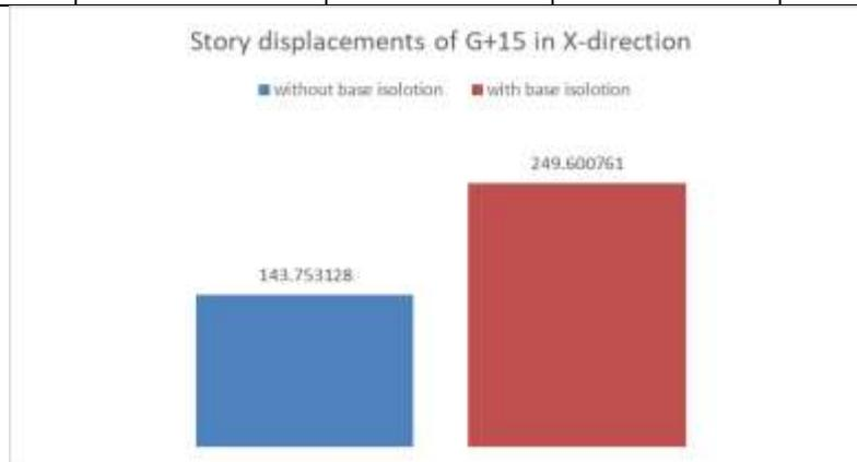
Fig 16: Story displacements of 15 stores in the x-direction
