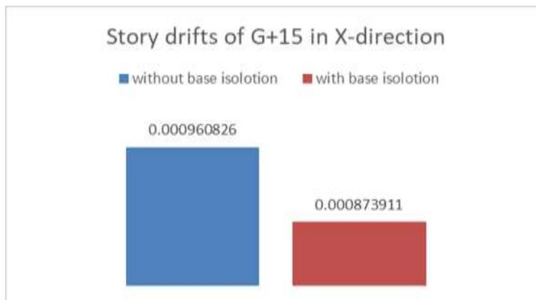
Fig 18: Story drifts of 15 stores in the x-direction
