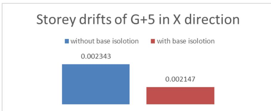
Fig 33: Story drifts of 5 stores in the x-direction
