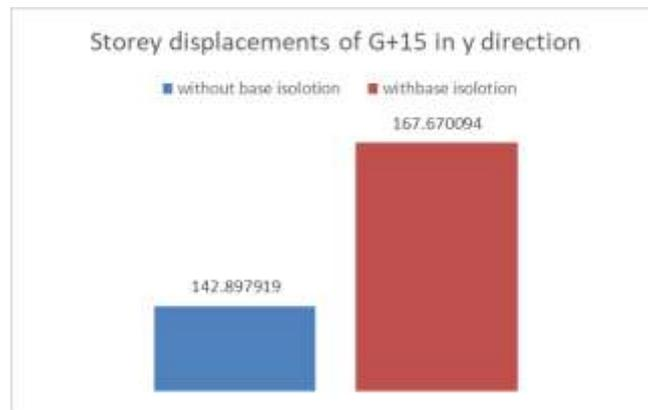
Fig 12: Story displacement of 15 stories in the y-direction
