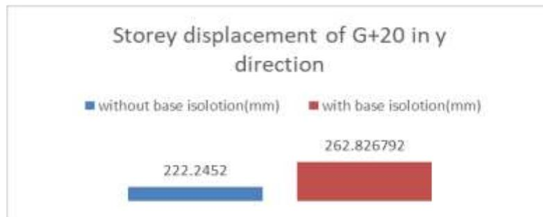
Fig 2: Story displacement of 20 stories in the y-direction
