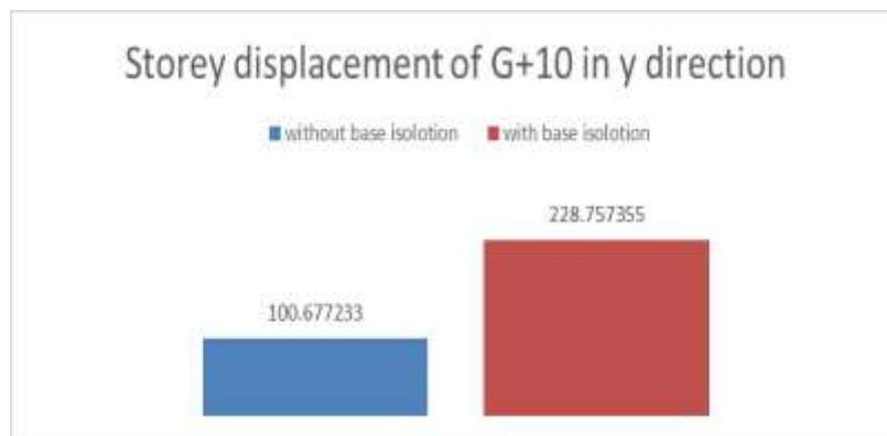
Fig 22: Story displacements of 10 stores in the y-direction
