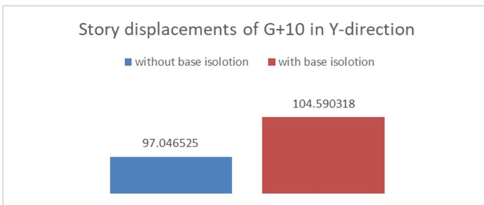
**Fig 27: Story displacements of 10 stores in the y-direction**
