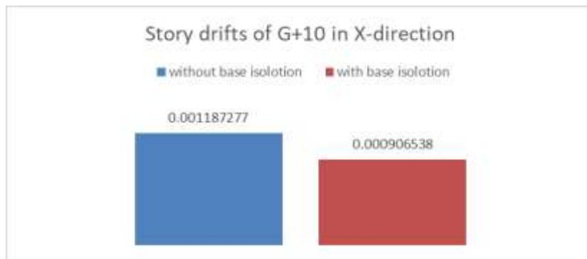
Fig 28: Story drifts of 10 stores in the x-direction
