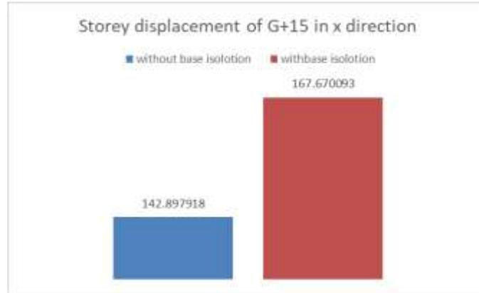
Fig 11: Story displacements of 15 stories in the x-direction
