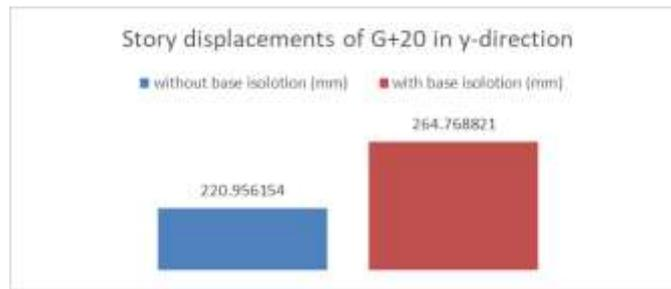
Fig 7: story displacements of 20 stories in the y-direction
