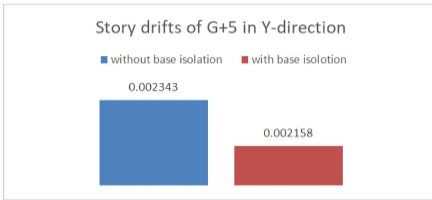
Fig 39: Story drifts of 5 stores in the y-direction
