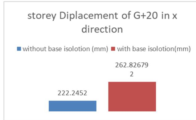
Fig 1: Story displacement of 20 stories in the x-direction
