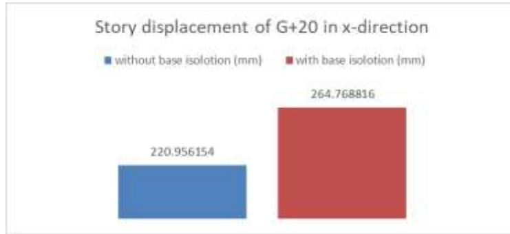
Fig 6: story displacements of 20 stories in the x-direction
