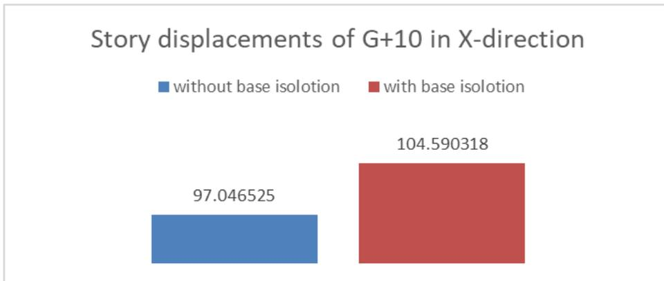
**Fig 26: Story displacements of 10 stores in the x-direction**
