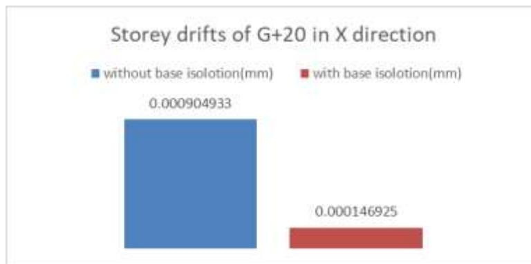
Fig 3: story drifts of 20 stories in an x-direction
