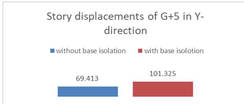
Fig 37: Story displacements of 5 stores in the y-direction
