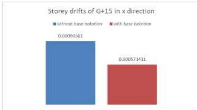
Fig 13: Story drifts of 15 stories in an x-direction
