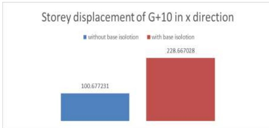
Fig 21: Story displacements of 10 stores in the x-direction
