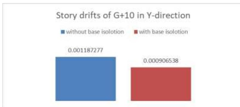
Figure 29: Story drifts of 10 stores in the y-direction
