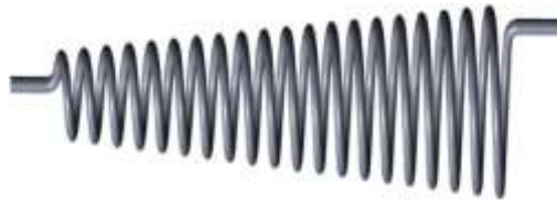
Fig 1. Cone helically coiled tube
