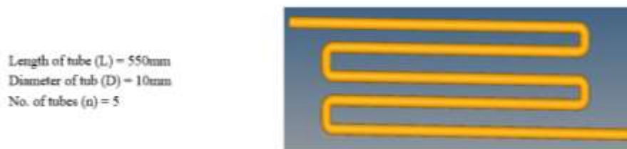
Fig. 2 - CAD model of radiator tubes
