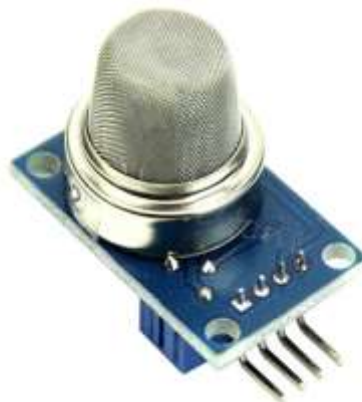
Fig. No. 4 Gas Sensor
