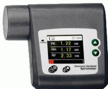
Figure 1: TeleBreather device that can be used at home to test how well patient's lung is working. (SHL Telemedicine, 2015)
