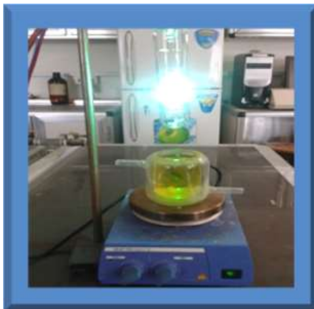
Fig. 1- Main parts of the photocatalytic cell used in Photocatalytic degradation of Malachite green dye.
