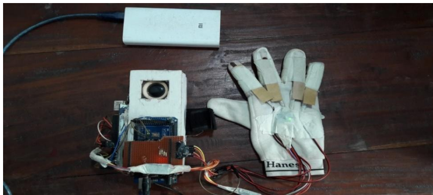
Fig. 2– Signs to speech converter
