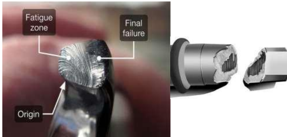
Fig 1. Fatigue zone and failure of the stainless steel material.
