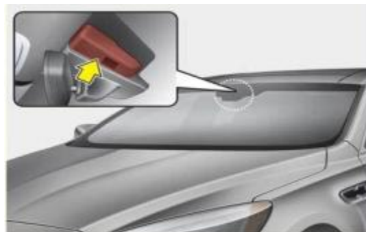
Fig.5 Automatic defog system [10]
