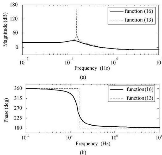
Fig.7. Bode diagrams of the transfer function between active power and power angle obtained with and without the current feedback loop.
