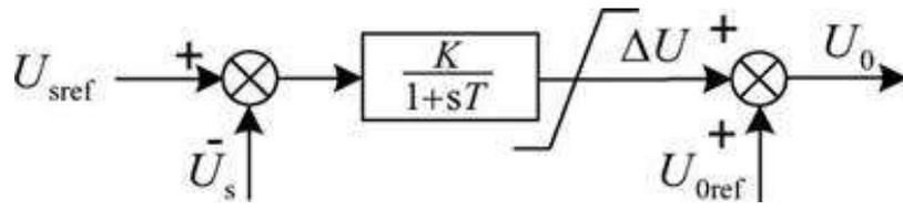
Fig. 6. AC voltage amplitude controller (AVAC)
