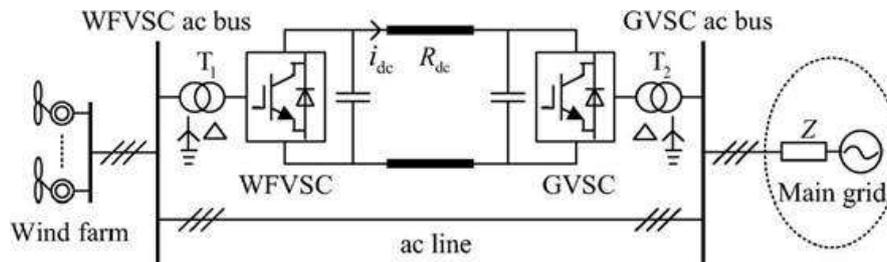
Fig. 1. Configuration of the wind farm grid connection via VSC-HVDC and ac hybrid transmission.
