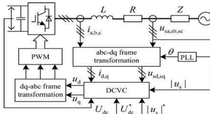
Fig .9. Schematic of the control system of GVSC.
