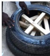
Plate 2: placing of wood in the tyre
