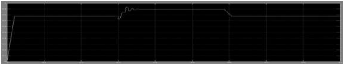
Fig 4.13.Voltage Vrms at load point, with three-phase fault , Without D-STATCOM
