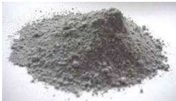
Fig.3 showing sample of Stone polishing waste
