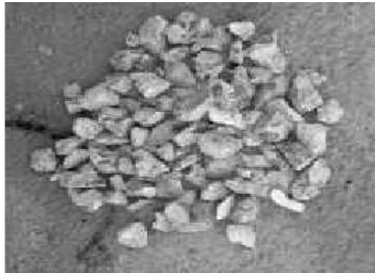
Fig.2 showing sample of recycled coarse aggregate
