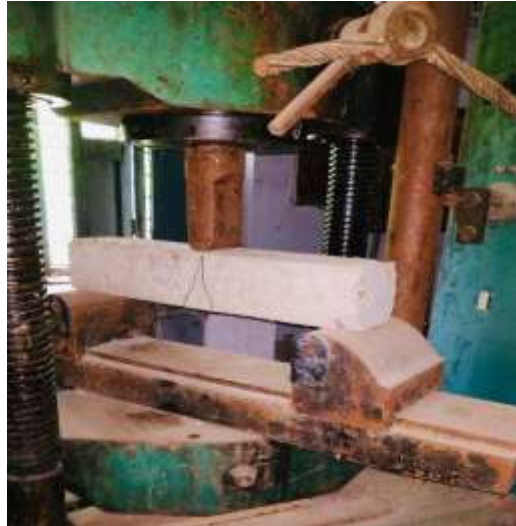
Fig.6 shows the testing of concrete prism.
