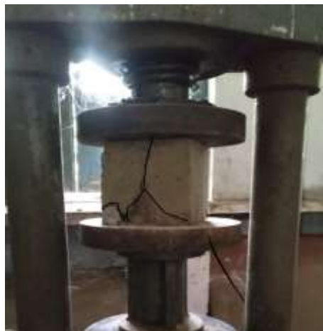
Fig.4 shows the testing of concrete cube for compressive test.
