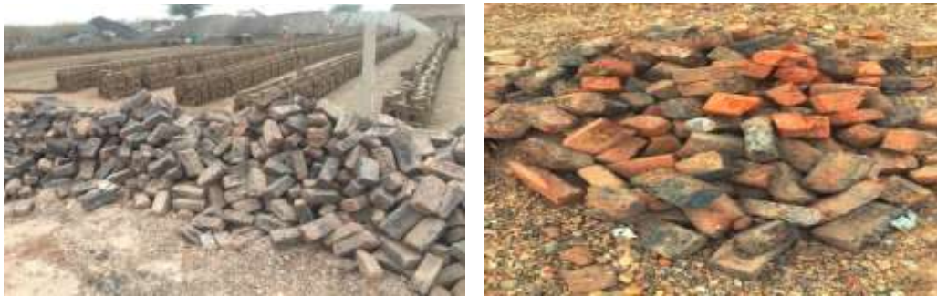
Fig.1 shows the over burnt bricks at manufacturing unit.
