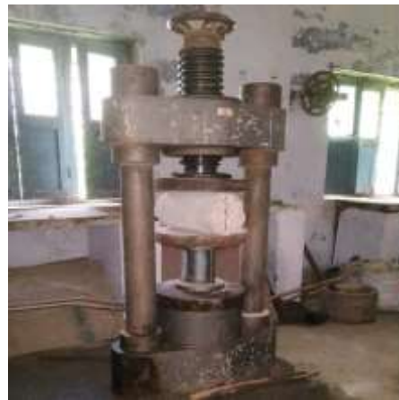
Fig.5 shows the testing of concrete cylinder for tensile strength test.
