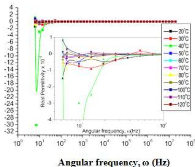
**Fig.10:** Plot of real component of permittivity against angular frequency of PANI-MnFe<sub>2</sub>O<sub>4</sub>-CTAB nanocomposite in RTILs.
