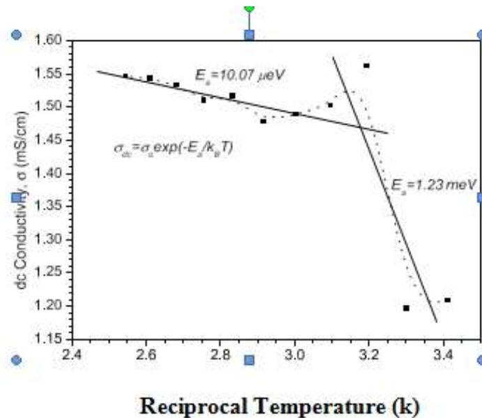
**Fig. 9:** Plot of dc conductivity against reciprocal temperature together with activation energies of the compound.
