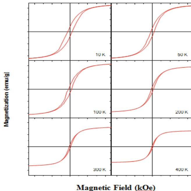
Fig.2: Hysteresis loops of PANI-MnFe<sub>2</sub>O<sub>4</sub>-CTAB nanocomposite at different temperatures
