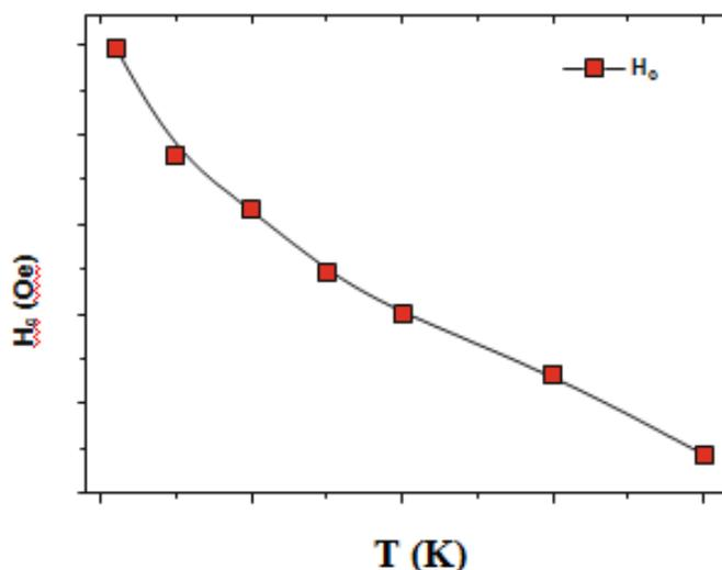
**Fig. 6:** Coercive field  $H_c$  as a function of temperature for PANI- $MnFe_2O_4$ -CTAB nanocomposite in RTILs
