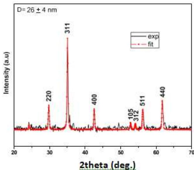
**Fig.1:** XRD powder pattern of PANI–MnFe<sub>2</sub>O<sub>4</sub>-CTAB nanocomposite.
