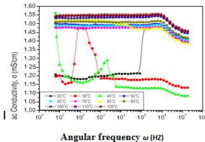
Fig. 8: Plot of ac conductivity of PANI-MnFe<sub>2</sub>O<sub>4</sub>-CTAB nanocomposite in RTILs at different temperature ranging from 20 to 120 °C from frequency range of up to 3 MHz.
