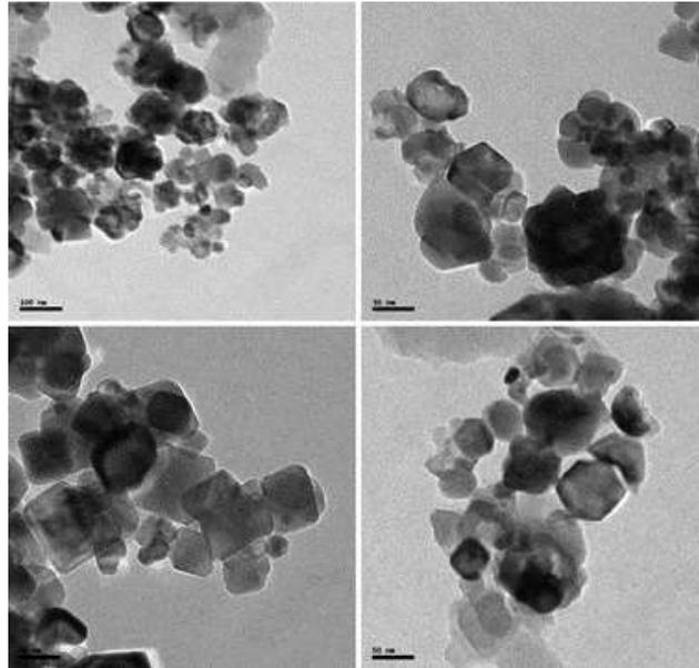
Fig.3: TEM Images of PANI-MnFe<sub>2</sub>O<sub>4</sub>-CTAB nanocompound with different magnification
