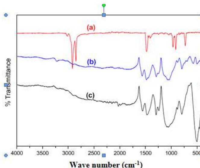
**Fig.2:** FT-IR spectra of (a) CTAB, (b) PANI and (c) PANI– MnFe<sub>2</sub>O<sub>4</sub>-CTAB nanocomposite.
