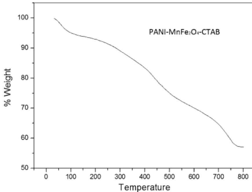
Fig. 7: TG thermogram of PANI-MnFe<sub>2</sub>O<sub>4</sub>-CTAB nanocomposite in RTILs
