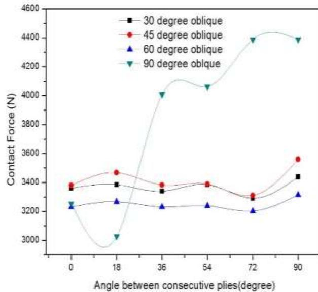
Fig. 3 Contact Force vs Angle between consecutive plies for different Oblique impact angles
