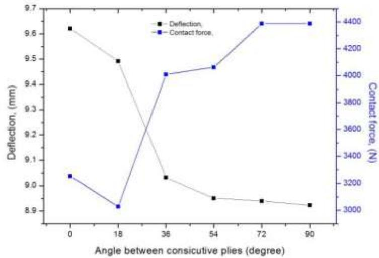
Fig. 2 Deflection and Contact Force vs. Angle between consecutive plies of carbon fiber composite laminate.
