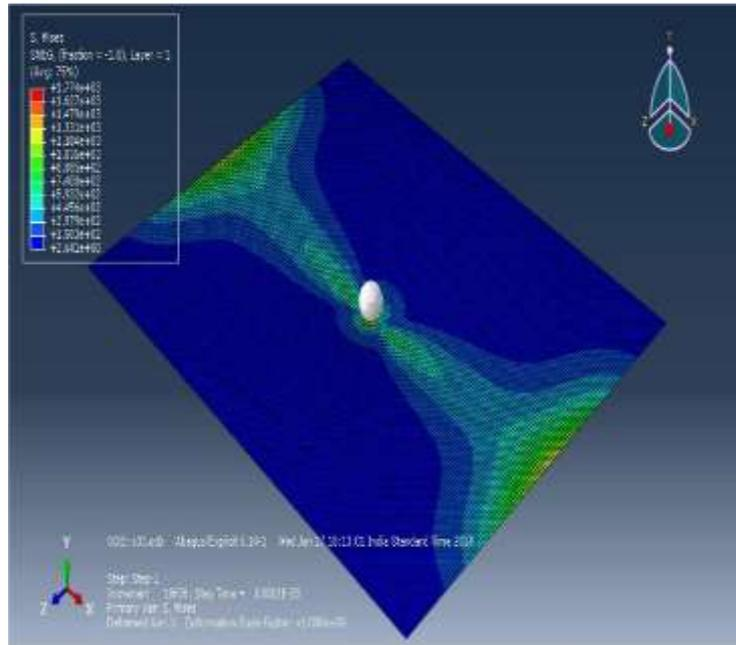
Fig.4 Stress contour under normal impact of 13.5J and fixed boundary conditions
