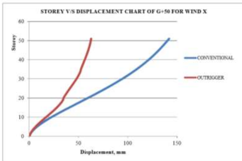
Fig. 6.14 Storey v/s displacement chart of G+50, for WIND X.
