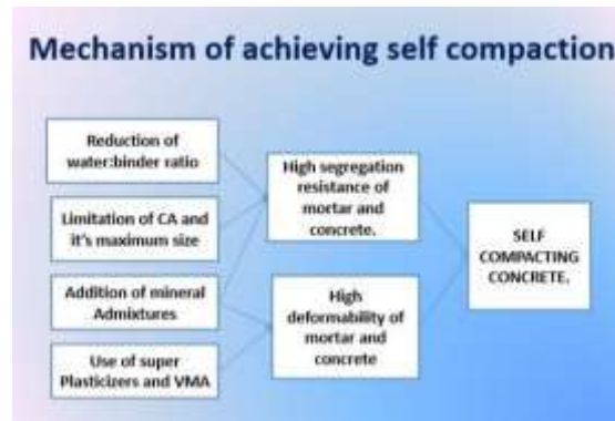
Fig. 4.1, Mechanism of Self Compacting Concrete
