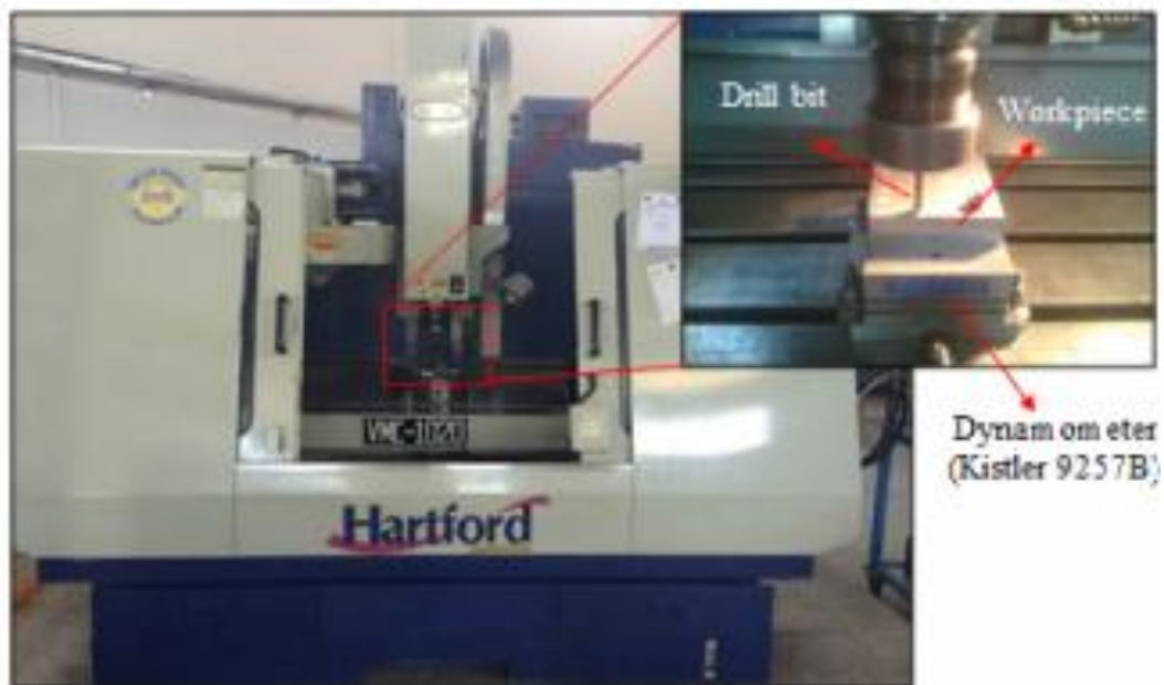
Fig 1. Drilling of composite material [10]
