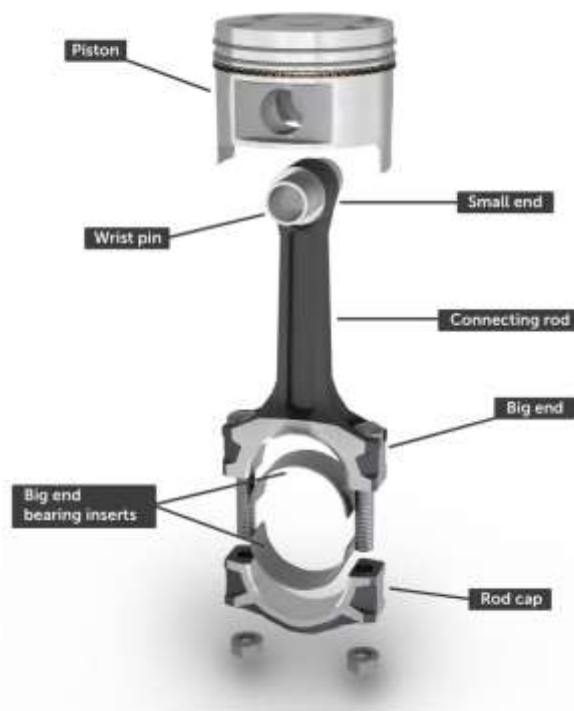
Figure 3 A connecting rod with nomenclature and piston
